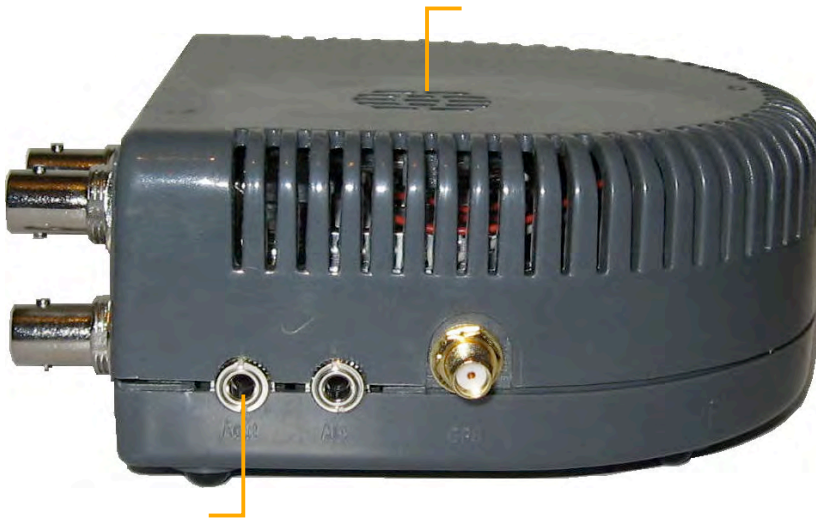
Figure 19: Internal speaker and Audio Out connector
