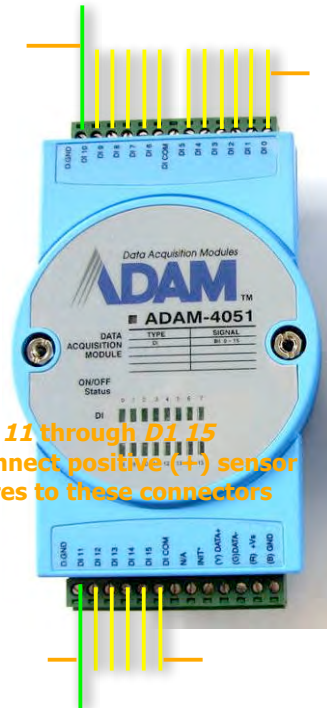
Figure 13: Connecting sensors to the ADAM-4051 module
