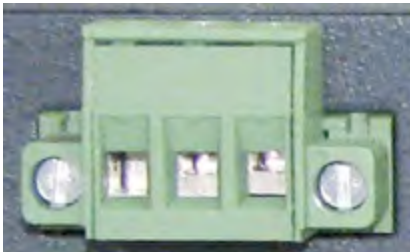
Figure 26: Wire connector plugged into Power connector
